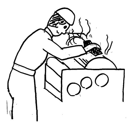
This sketch illustrates an example of occupational exposure to 1,2-dichloropropane, a solvent that is used for cleaning offset printing presses. Unprotected workers who clean the printing machines by hand are exposed to high levels of 1,2-dichloropropane vapour at close proximity, particularly in small, poorly ventilated rooms. This type of specific and intense exposure to 1,2-dichloropropane was observed in epidemiological studies on which the Working Group based its evaluation.
